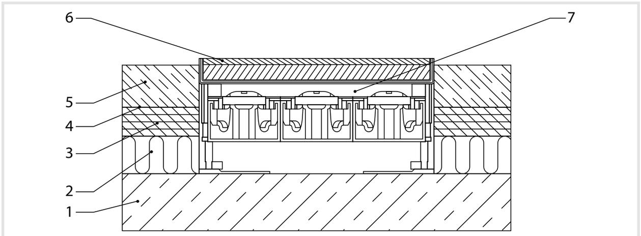
Figure 5: Concept drawing of the stainless steel cassette EKQ1200LE1 test setup in the ceiling test station
