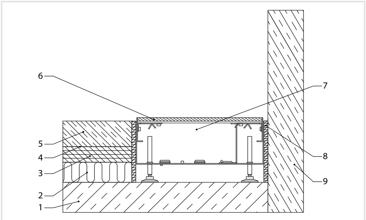
Figure 3: Concept drawing of the floor channel BKB25085 test setup in the ceiling test station
