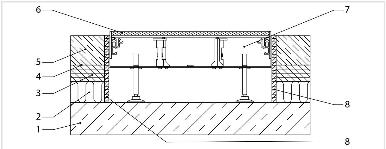
Figure 4: Concept drawing of the floor channel BKG30060 test setup in the ceiling test station
